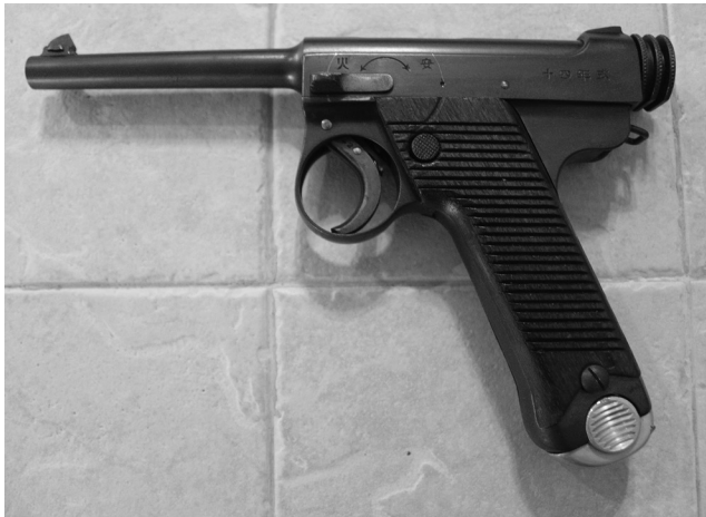
Figure 5.12 A wartime Japanese Type 14 pistol, but simply known as the "Nambu," a generic term for the series of pistols of this design. The basic design mimics the Luger or Lahti pistol. (Image from author's collection.)
